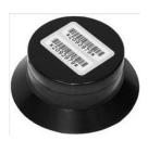
The sampler has a piece of plastic inside that can be marked by alpha particles in the air. The marks can be counted with a high power microscope.
