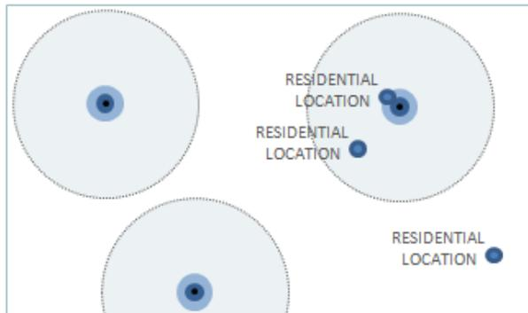
A geographic information system was used to overlay residential locations (represented by street block centre points) with the modelled or estimated concentration gradients of industrial emitters.
